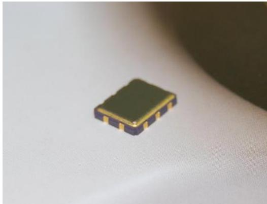
**Low Loss SAW 286.2 MHz Filter**
