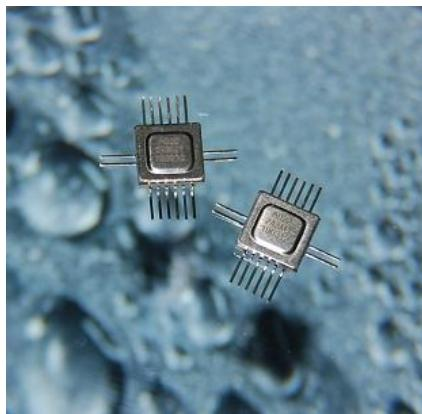
**Low Loss SAW 263 MHz Filter**
